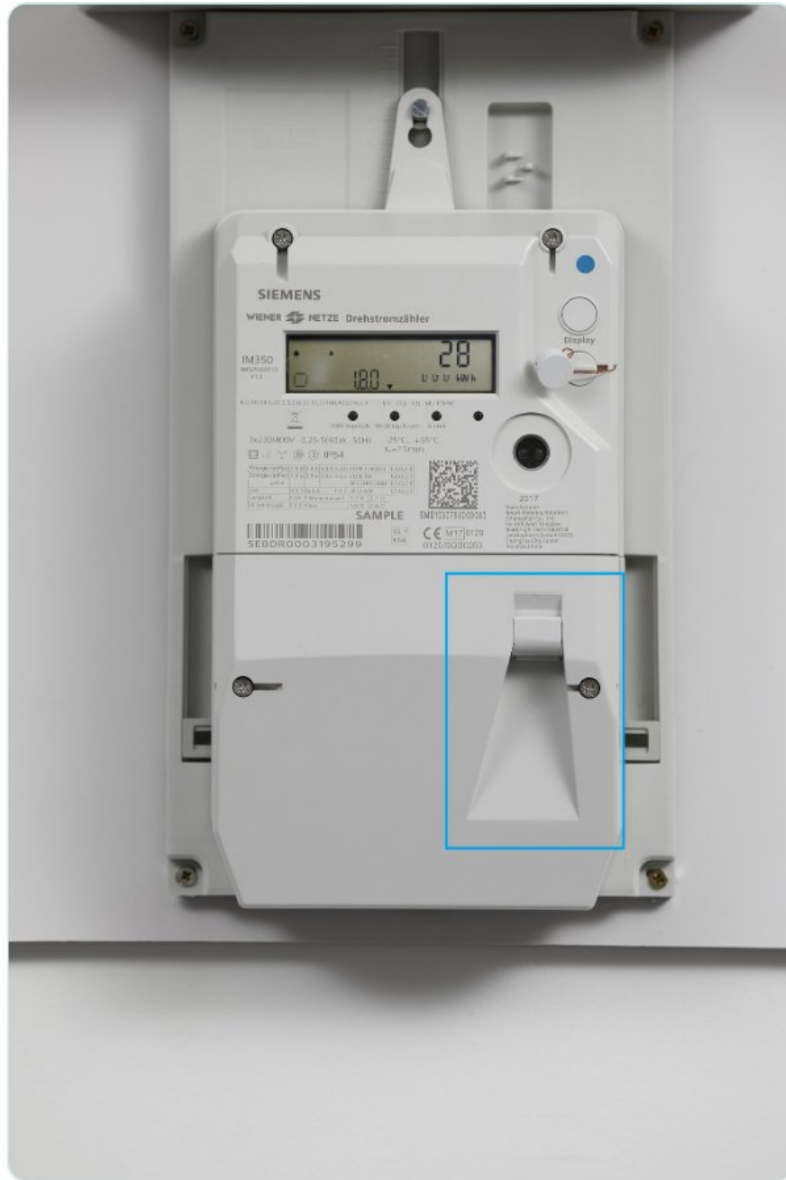
PI port on the Siemens IM350
