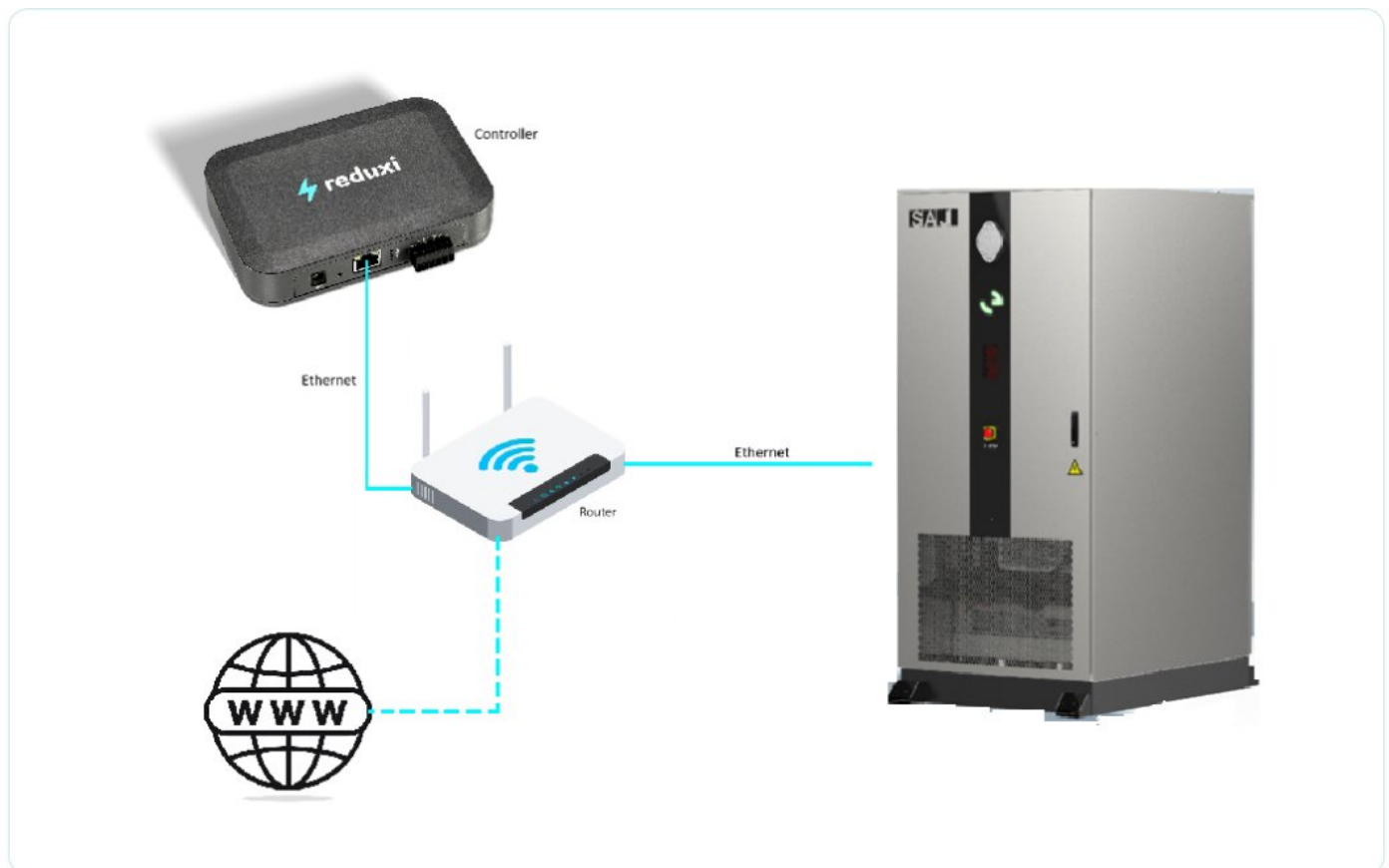
Physical connection of the SAJ CM2 and the Reduxi Controller
