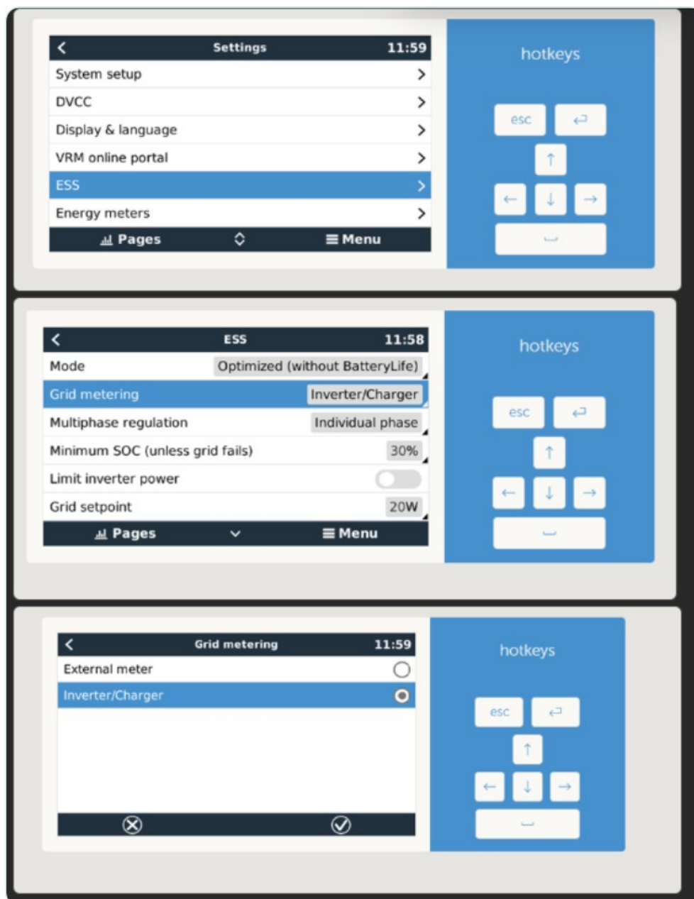
ESS settings: Settings – ESS, then Grid metering
