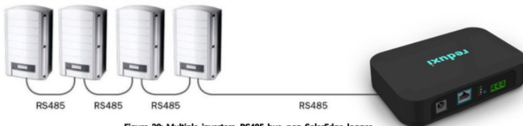
Figure 20: Multiple inverters, RS485 bus, non-SolarEdge logger
