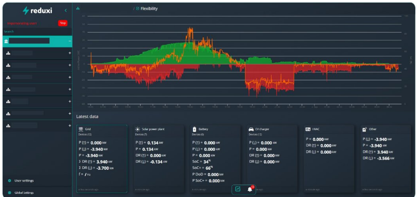
Aggregator account main view: location navigation with Global Settings , flexibility chart and device overview
