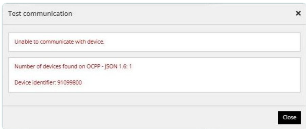
Test communication: the window lists the chargers connected via OCPP and their device identifiers
