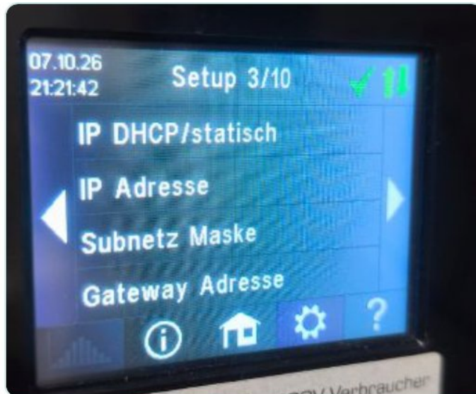
Setup 3/10 – network settings on the display
