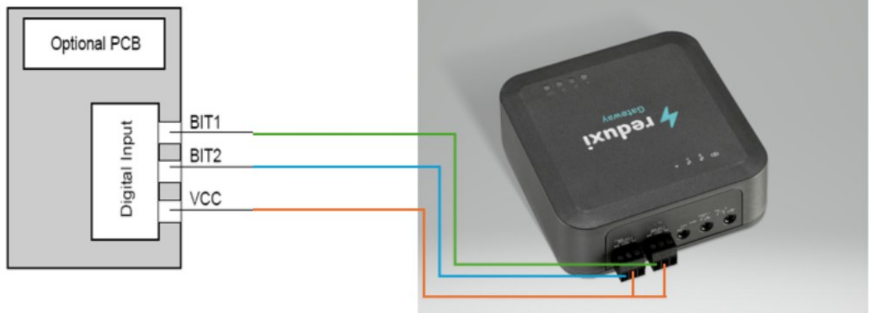
Connection of the relays to the SG-ready contacts
