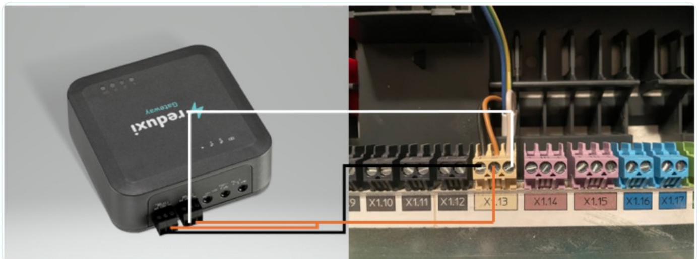
Connection from the Reduxi Gateway device to the SG-ready contacts
