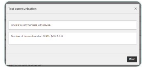
Case 3: No device with OCPP 1.6 communication is found
