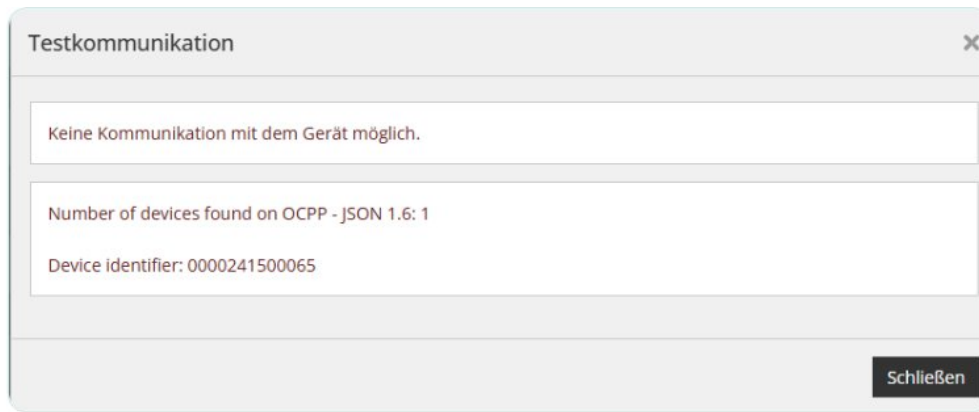
Case 2: ID of device is not set or is different
