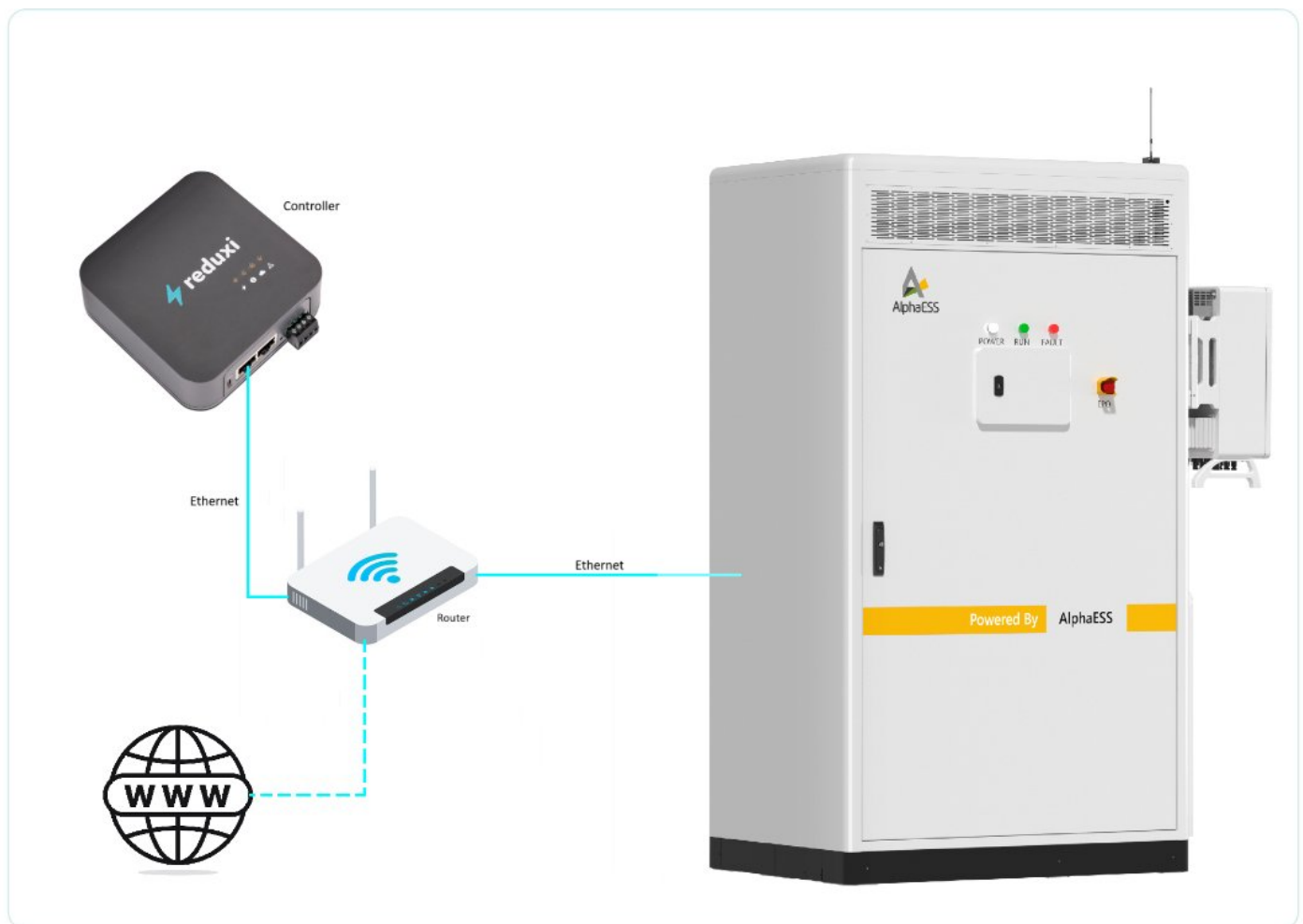
Connection from the Reduxi Controller to the AlphaESS system
