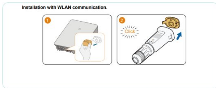
Installation with WLAN communication
