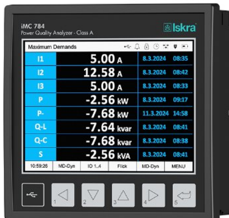
Iskra iMC784 power quality analyzer
