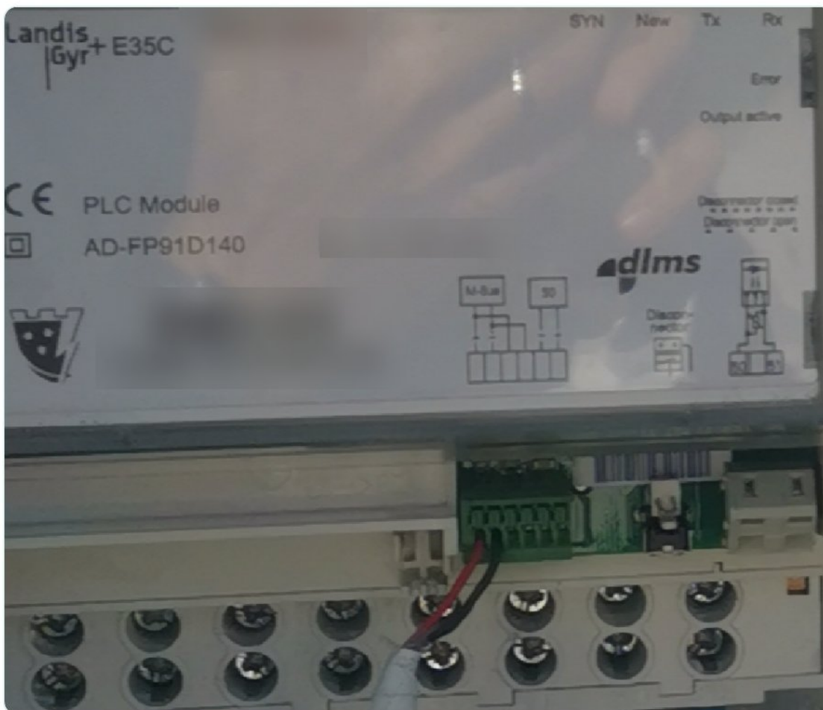
M-Bus pins on the energy meter
