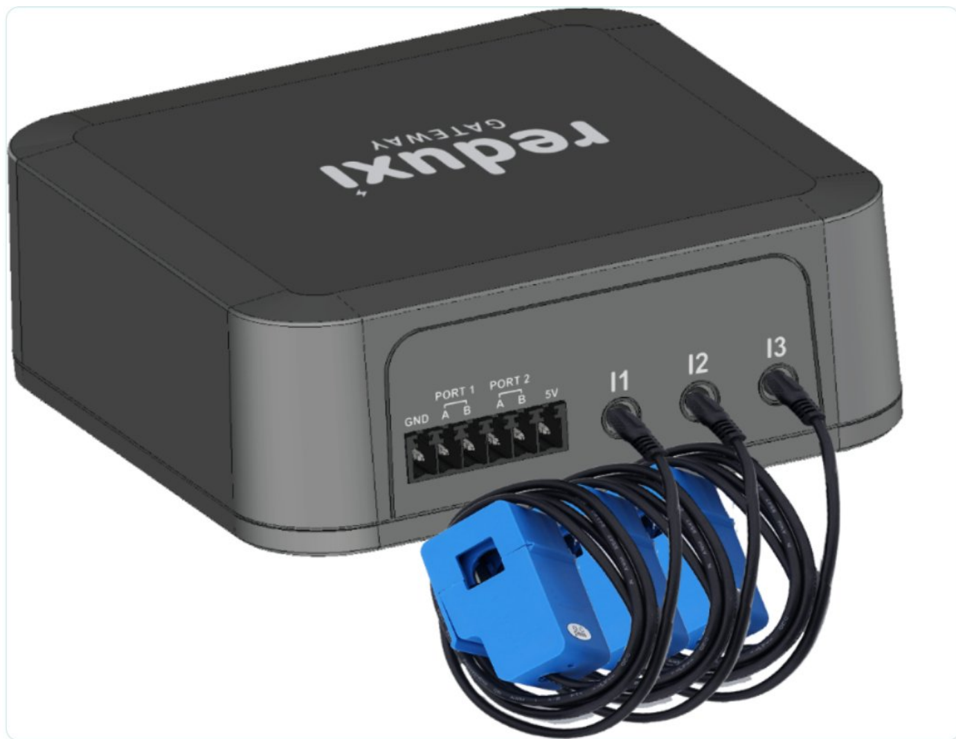
Current sensors connected to the Reduxi Gateway
