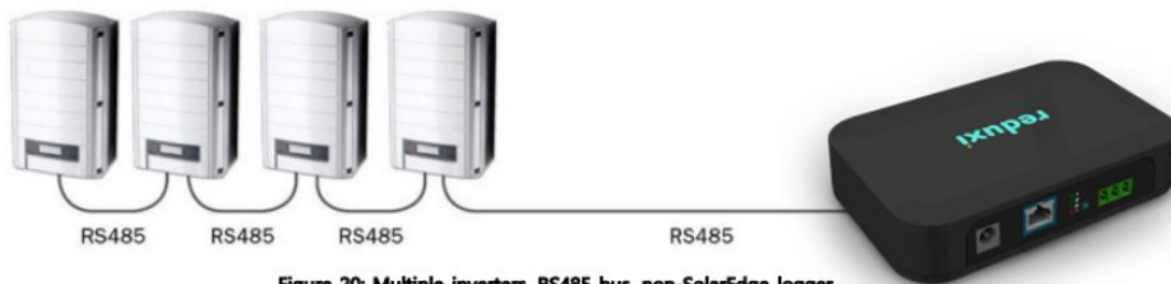
Figure 20: Multiple inverters, RS485 bus, non-SolarEdge logger
