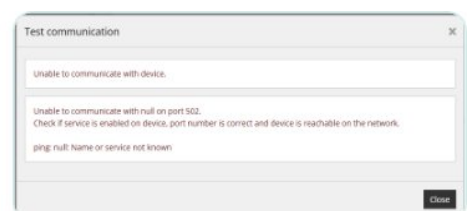
2. Failed test: the system is not configured correctly
