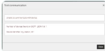
Case 2: Unable to communicate with device 1, ID of device is not set or is different
