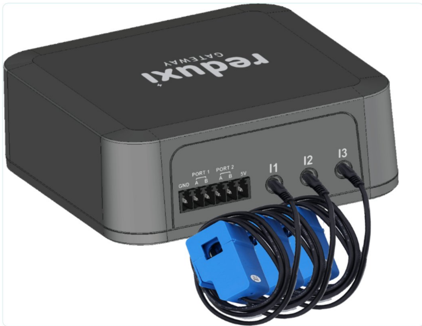
Current sensors connected to the Reduxi Gateway
