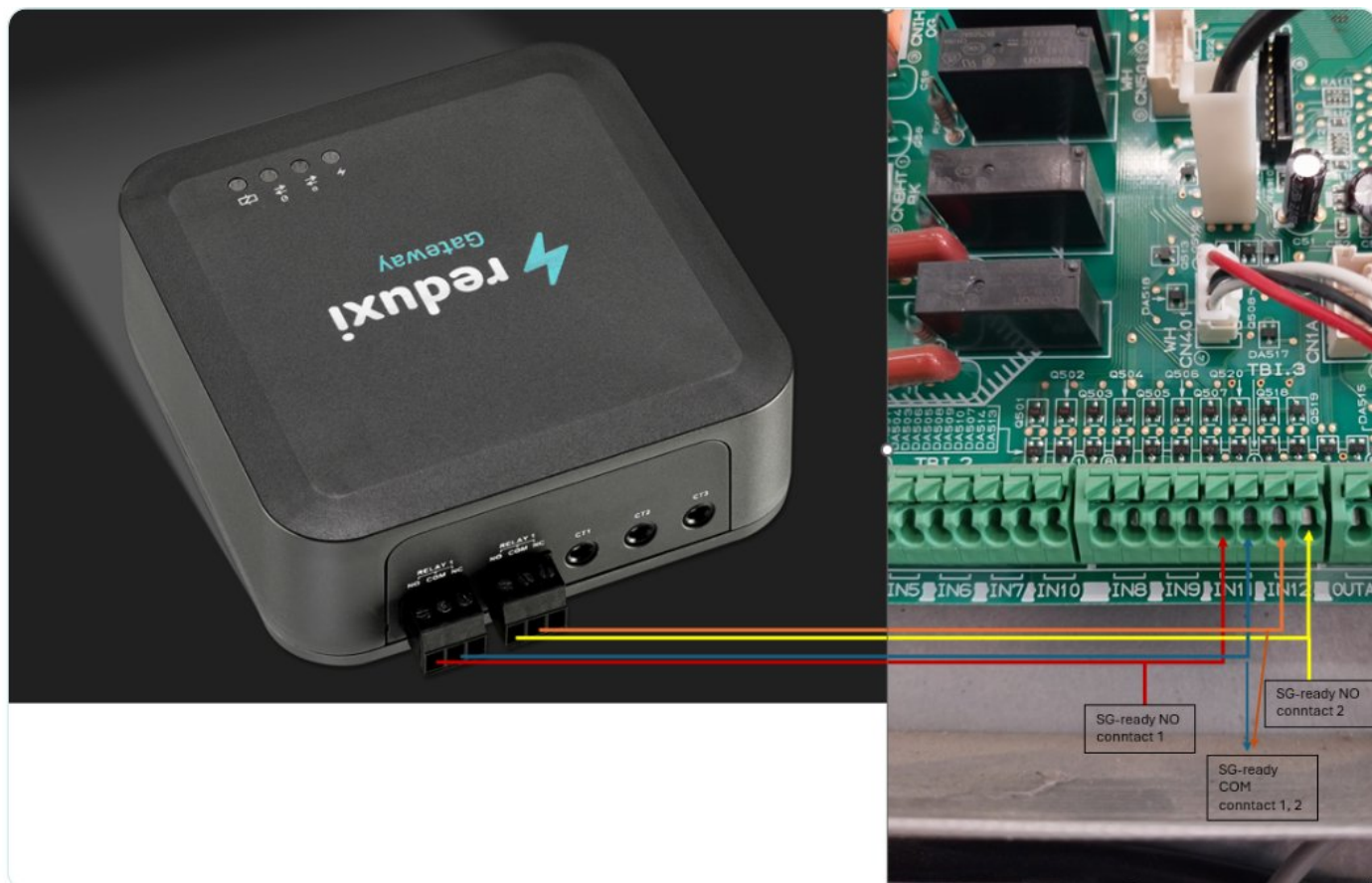
SG-ready contacts of the Ecodan connected to the Reduxi Gateway
