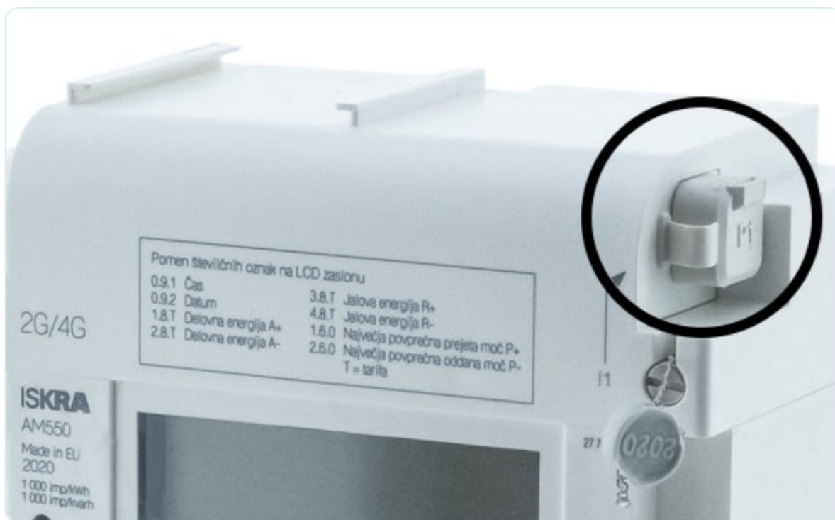
P1 port in the upper right corner of the Iskraemeco AM550
